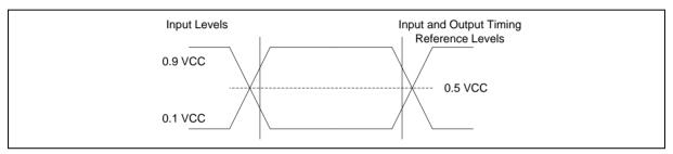
Figure 36. AC Measurement I/O Waveform
