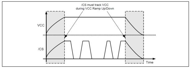
Figure 35b. Power-up, Power-Down Requirement
