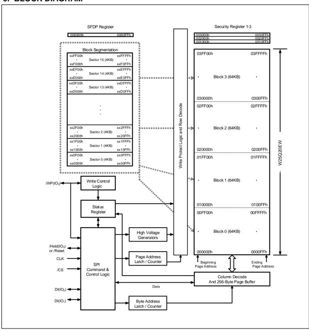
Figure 2.W25Q20EW Serial Flash Memory Block Diagram
