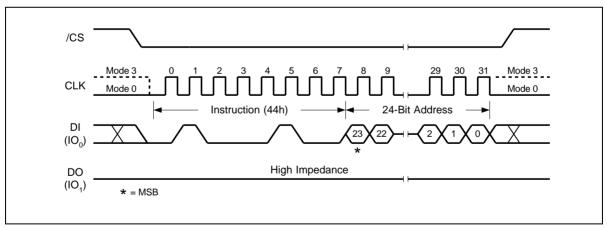
Figure 35. Erase Security Registers Instruction Sequence(SPI mode only)
