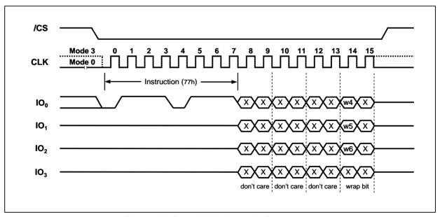
Figure 15. Set Burst with Wrap Instruction Sequence
