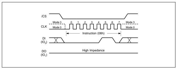
Figure 4. Write Enable Instruction Sequence Diagram
