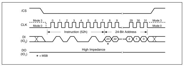
Figure 20. 32KB Block Erase Instruction Sequence Diagram
