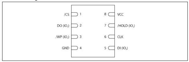
Figure 1b.W25Q20EW Pad Assignments USON 2x3-mm (Package Code UX)
