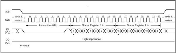
Figure 8. Write Status Register Instruction Sequence Diagram
