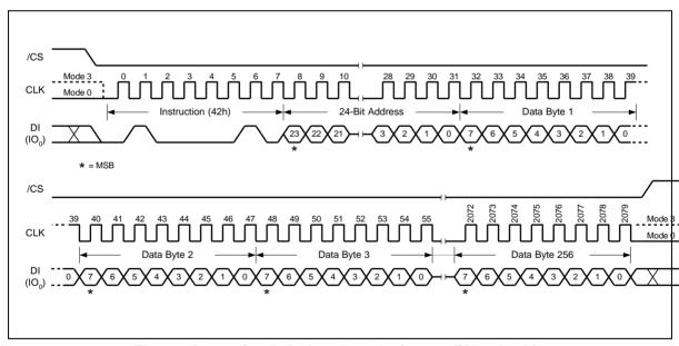
Figure 36. Program Security Registers Instruction Sequence(SPI mode only)
