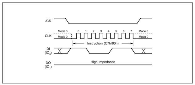
Figure 22. Chip Erase Instruction Sequence Diagram
