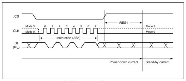
Figure 26a. Release Power-down Instruction Sequence
