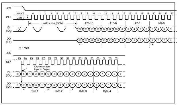
Figure 13a. Fast Read Dual I/O Instruction Sequence (Bits M7-0 must be set to FFh)
