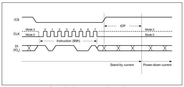
Figure 25. Deep Power-down Instruction Sequence Diagram
