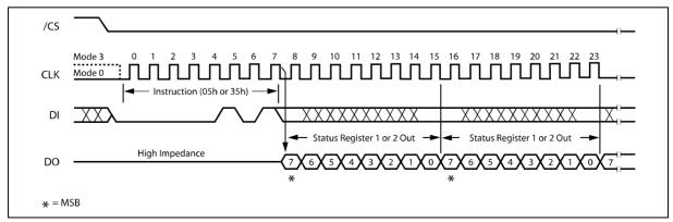
Figure 7. Read Status Register Instruction Sequence Diagram
