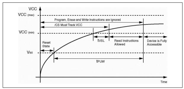
Figure 35a. Power-up Timing and Voltage Levels
