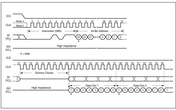
Figure 10. Fast Read Instruction Sequence Diagram
