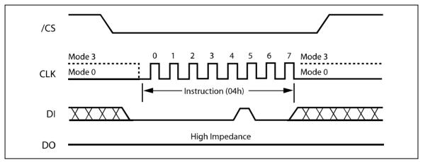
Figure 6. Write Disable Instruction Sequence Diagram
