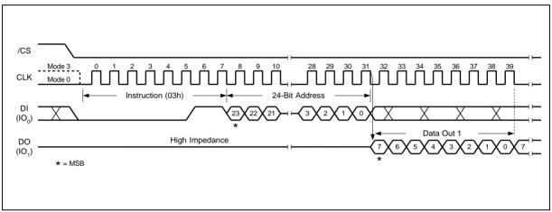
Figure 9. Read Data Instruction Sequence Diagram
